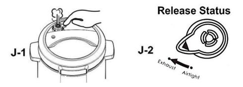
When enough pressure has been released, the cover (lid) will be unlocked from the main body of the unit and can then be removed.
