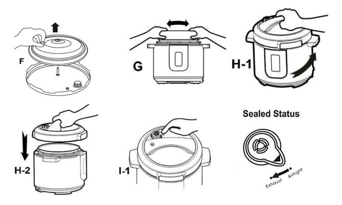
**Note:** The exhaust valve (steam release valve) does not click or lock into place. Even though it will have a loose fit, it is safely secured.
