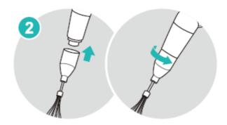
Insert the whisk adaptor into the motor body and twist to lock until it clicks.
