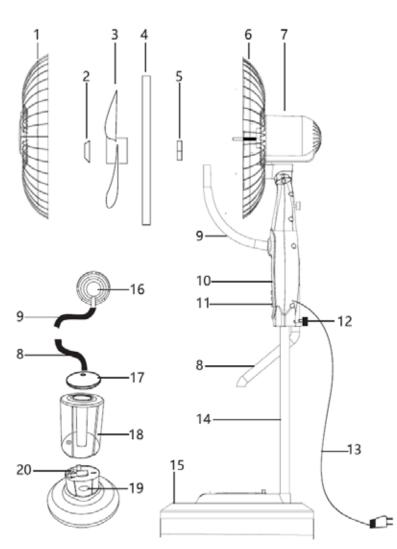
1.Front grid 2.Blade spinner 3.Blades 4.Net frame 5.Plastic nut 6.Rear grid 7.Motor 8.Lower flexible hose 9.Upper flexible hose 10.Function indicators 11.Control buttons 12.Bolts 13.Power cord 14.Supporting tubes 15.Base and base cover 16.Mist vent (front grid) 17.Water tank cover 18.Water tank 19.Water tank indicator 20.Mist generator
