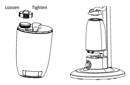
Unscrew the valve cover to open the tank turning it anticlockwise, fill the tank with cold and clean water making sure not to overfill it. To close the tank, screw the valve cover back on securely turning it clockwise. Turn the tank over and place it back into its designated space at the back of the fan main body.
