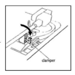
Push the Lift Lever up to raise the Tone Arm and then gently move the Tone Arm to the desired position over the record.
